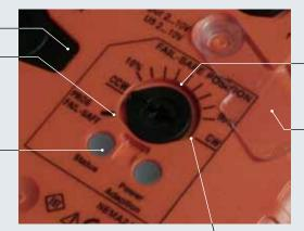
0...100% intermediate positions in step of 10% from front panel.
